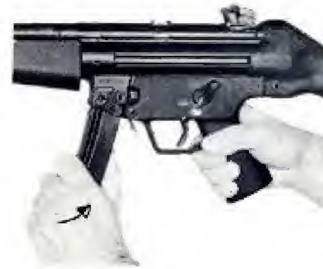
Fig. 27 Inserting the magazine
